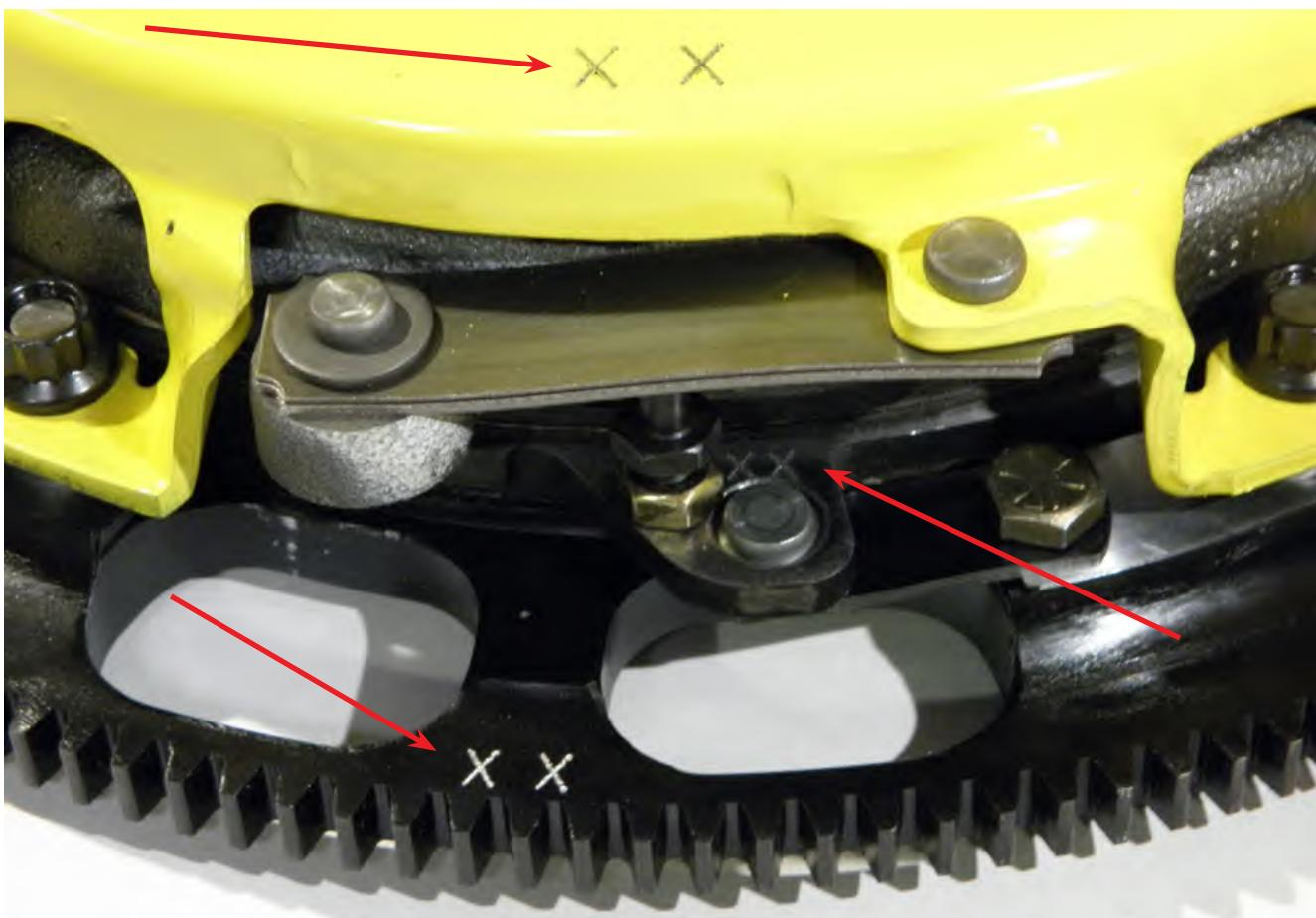
8. The adjustment feature of the floater plate is highly critical to the correct function of the clutch. If you wish to check the adjustment, see the "Adjustment" section for more information.
