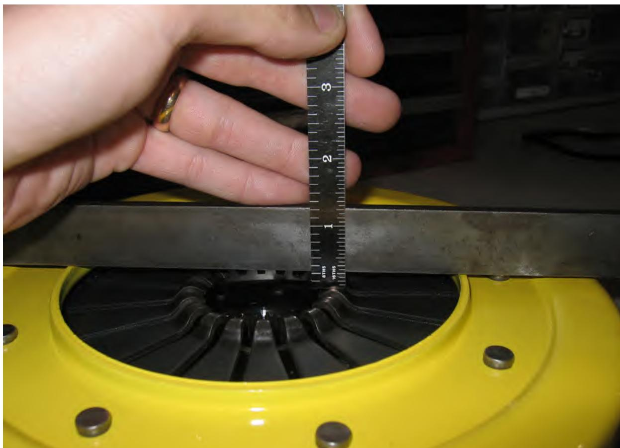
**Warning:** If you change the amount of pressure plate shims or change components, you must readjust floater lift. Otherwise the clutch will not release properly and you risk damage to the assembly or possibly your transmission.
