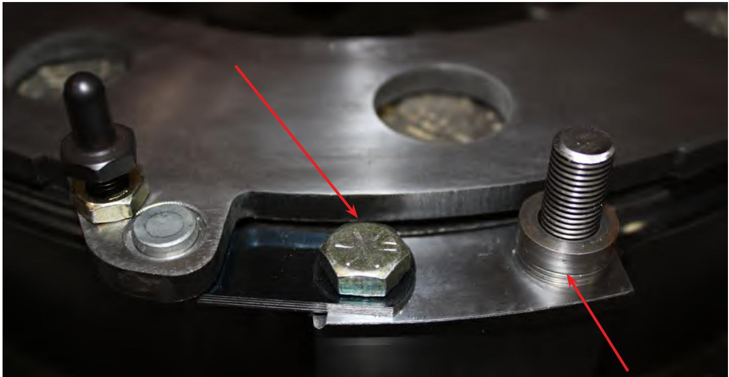
NOTE: For your convenience when purchased as a complete kit, the floater lift is preset by ACT for new installation and separate components are marked for position. For more information see the "Adjustment" section.
