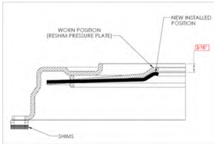
**Floater lift adjustment:** Once all the components are installed onto the engine and the pressure plate is shimmed and tightened down you can adjust for floater lift. First loosen the jamb nut located at the bottom of the floater adjustment stud then screw the floater adjustment stud away from the pressure plate drive straps. Adjust as described below.
