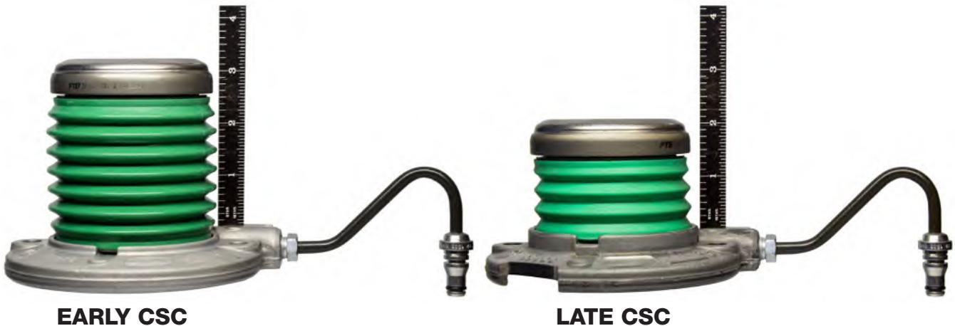
The **EARLY** CSC measures approximately **3-1/4" / 82.5mm** and the **LATE** CSC is **2-1/8" / 54mm**. **IF USING THE LATE CSC, THE SPACER INCLUDED IN THE KIT MUST BE INSTALLED. DO NOT INSTALL THE SPACER IF USING THE TALLER CSC!**
