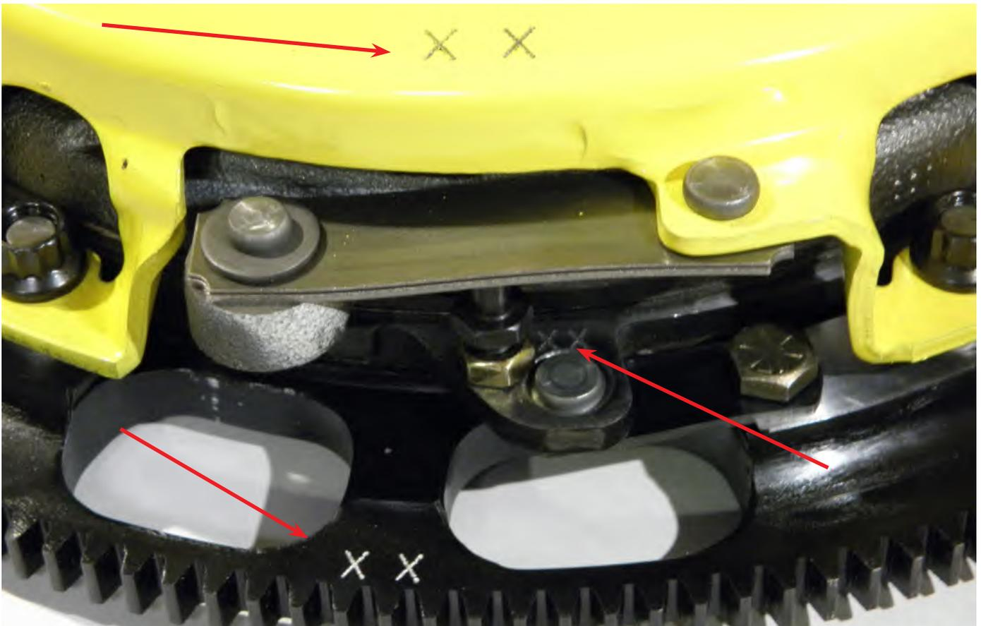
8. The adjustment feature of the floater plate is highly critical to the correct function of the clutch. If you wish to check the adjustment, see the **Adjustments** section (page 4) for more information.
